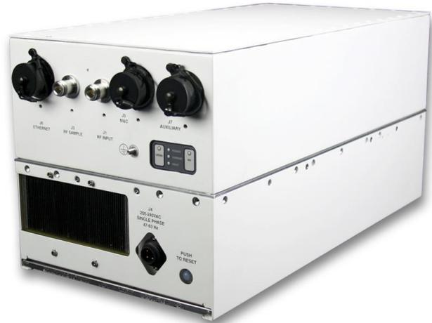
The PA20-Ka500 series power amplifiers provide the best in class Size, Weight and Power performance of any SATCOM outdoor power amplifier. These amplifiers are designed to optimize linear power performance and minimize power consumption, making them the most efficient linear power amplifiers available. The carbon footprint of a PA20-Ka500 is driven by the high efficiency power conversion of the traveling wave tube; an unmatched technology for power conversion.
